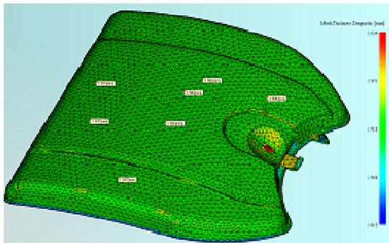
Above is a typical 3D mesh as used in both flow simulation and stress analysis packages to replicate an actual moulded part. Rosti have saved its customers significant development cost, material cost and lead time to market. Major projects can now have little or no prototyping expenses and go directly to "Hard tooling".
