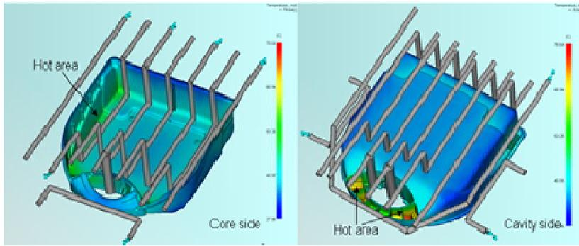
Above is a typical analysis of cooling efficiency. This advanced modelling will ensure: stable geometry of the moulded part and an optimised cycle time for competitive cost.
