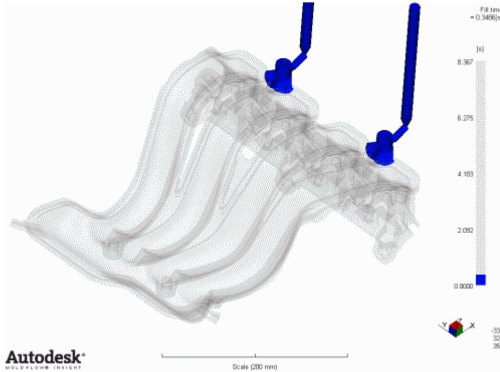
The complex automotive component above is an innovation. It is one piece of a two piece plastic inlet manifold system. Earlier generations of this assembly used more components to eliminate the complex geometry and avoid mould-ability issues. Rosti accepted the challenge of optimising the customer's concept and developing ground breaking tooling to deliver the system on time.
